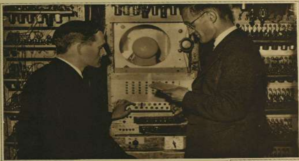
A CALCULATING MACHINE WITH A "MEMORY": THE CONTROL PANEL, AND A STORAGE TUBE IN USE
